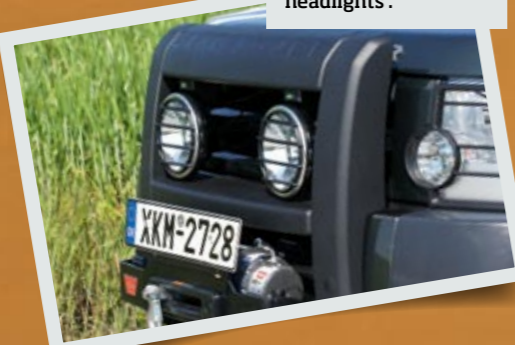
Bullbar with auxiliary headlights.
