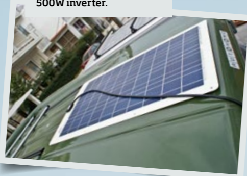
75W solar panel by Conergy provides 220V electricity through an auxiliary 45A dry type battery and a 500W inverter.
